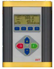
All instrumentation measurements are made using high accuracy voltage and current transformers located within the load bank. This information is processed. Digitally, using high-speed sampling of the raw data; this provides full three-phase true rms measurements with high update rates.
